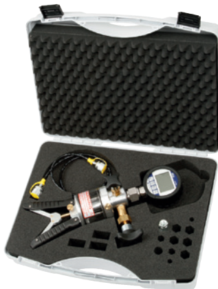
Basic version incl. hydraulic pressure generation
